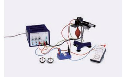
Charged oil droplets subjected to an electric field and to gravity between the plates of a capacitor are accelerated by application of a voltage. The elementary charge is determined from the velocities in the direction of gravity and in the opposite direction.
