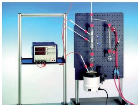
Crude oil, still one of the most important raw materials in the world, is a mixture of many hydrocarbons. Because the crude oil is a mixture of substances with different boiling temperatures, individual substances with different boiling ranges can be separated by distillation in fractions. In this experiment a model of crude oil is distilled.
