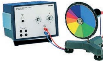
If a circular disc separated into various differently coloured sectors is rotated by a motor so fast that the eye can no longer distinguish the colours, a mixed colour is then perceived. By varying the composition and size of the sectors, it is possible to give the impression of any colour at all. The colour triangle can be used to predict what the perceived colour will be.
