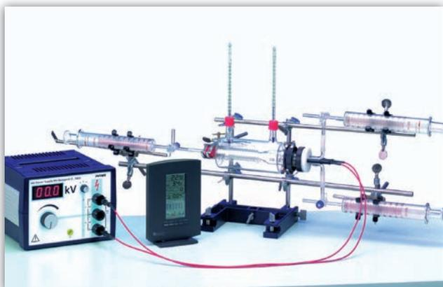
Energy balances at gas reactions (e.g. Determination of the heat of formation of water, P3021501)
