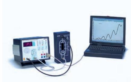
Electrons are accelerated in a tube filled with neon vapour. The excitation energy of neon is determined from the distance between the equidistant minima of the electron current in a variable opposing electric field.
