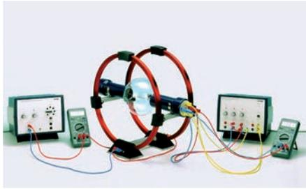
Electrons are accelerated in an electric field and enter a magnetic field at right angles to the direction of motion. The specific charge of the electron is determined from the accelerating voltage, the magnetic field strength and the radius of the electron orbit.
