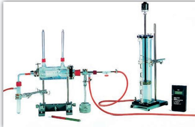
Calorimetry (e.g. Determination of calorific value of coal, P3021601)
