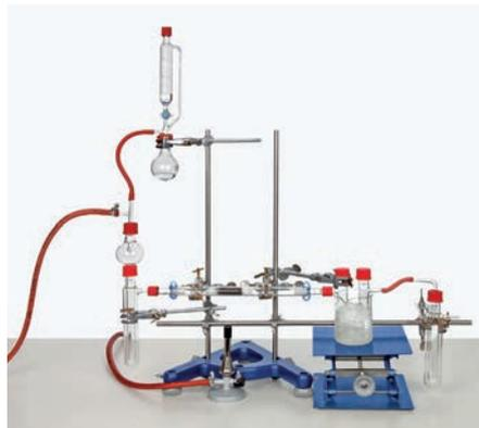
The contact process is currently used in the chemical industry to produce sulphuric acid in the high concentrations needed for industrial processes. In this model experiment, platinum-palladium-aluminium-oxide beads are employed as a catalyst for the reaction.
