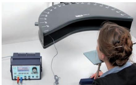
As excitation of the light-perceptive cells of the retina always takes a little longer than the light stimulus, only a limited number of stimuli per unit of time can be processed (time-related resolving power of the eye). If a light source is switched on and off periodically in increasingly rapid sequence the eye at first perceives the individual flashes, then the appearance of flicker occurs and finally the impression of a continuous light (fusion of the flicker).
