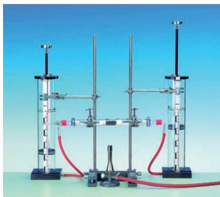
In this experiment the composition of air is investigated. Therefore solid copper is heated on air. Copper combines with the oxygen of air and forms copper oxide. If this reaction is performed in a closed apparatus and the air volume is measured before and after the experiment, the difference of the measured volume shows the oxygen content of the air.
