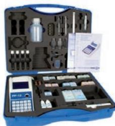
This excursion case enables students to actively participate in the measurement of water parameters in your immediate neighbourhood. Rapid chemical analyses provide meaningful results in a very short time. The colourimetric tests can be reproducibly and exactly evaluated by using the portable filter photometer.
