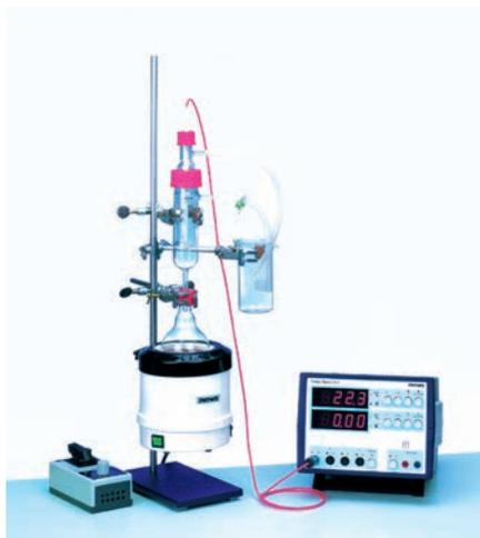
The boiling point of a solution is always higher than that of the pure solvent. The dependence of the temperature difference (elevated boiling point) on the concentration of the solute can be determined using a suitable apparatus.
