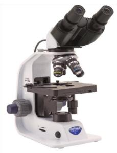
Binocular microscope, 1000x, HC objectives, with Automatic Light Control
