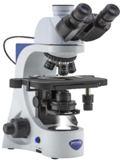
*Binocular brightfield microscope, 1000x, IOS N-PLAN objectives, with Automatic Light Control*
