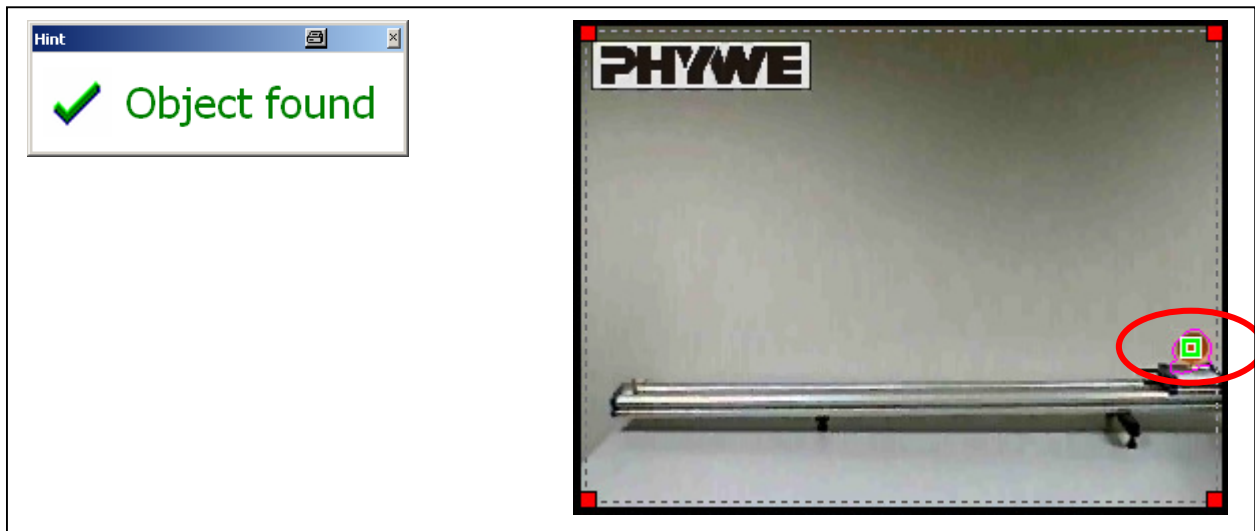
Fig. 18: Automatic analysis: the preliminary examination algorithm has recognized a moved object at this point.
