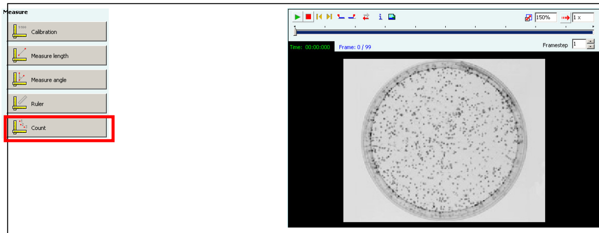
Fig. 25: Counting using the example of colony counting, i.e. counting cell colonies in a Petri dish.
