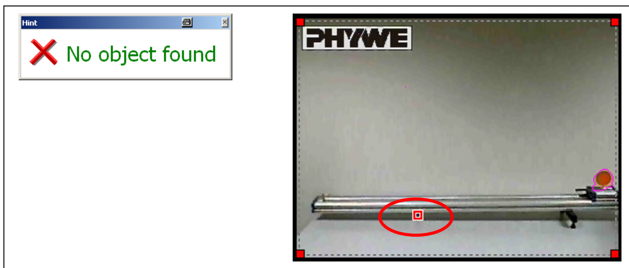
Fig. 19: Automatic analysis: the preliminary examination algorithm has not recognized a moved object at this point (!)
