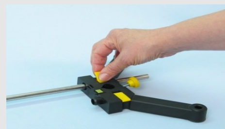
Fixing the stand rod
