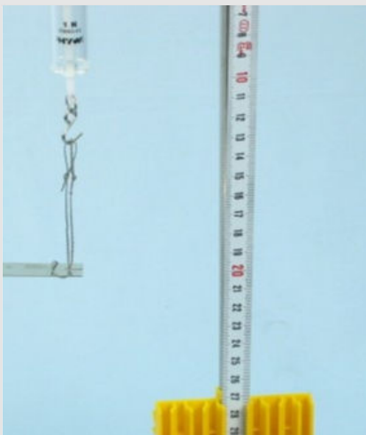
Connecting force gauge and leaf spring
