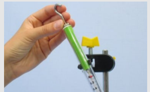
Inserting and adjusting the force gauges
