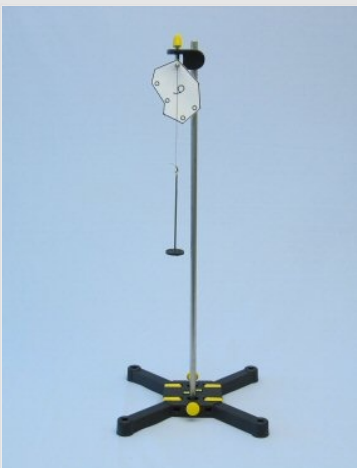
Lot method for determining the centre of gravity
