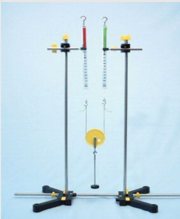
Test set-up for determining the force on a loose pulley
