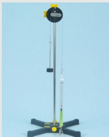
Test setup for determining the acting force
