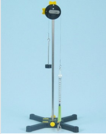
Test setup for determining the acting force
