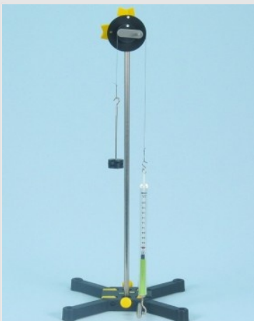
Test setup for determining the acting force
