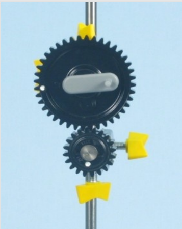
Test setup of the single-stage gear transmission
