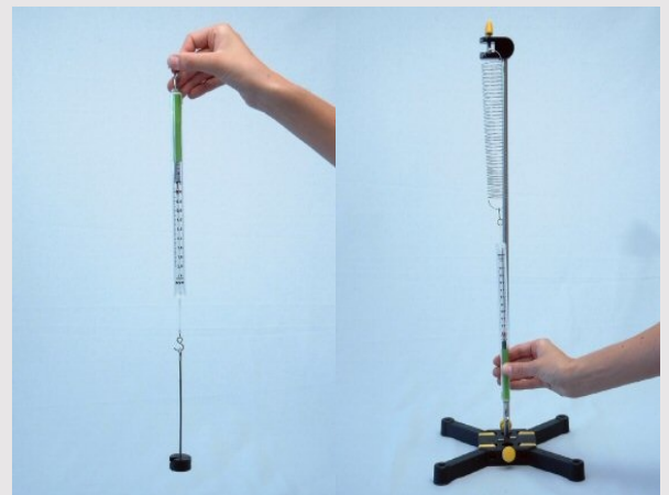
Lifting a mass and stretching a spring, each with the aid of a force gauge
