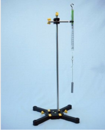
Determination of the weight forces in air F_{W,Air}
