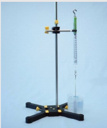
Experimental set-up for determining the density of a body by means of its buoyancy force
