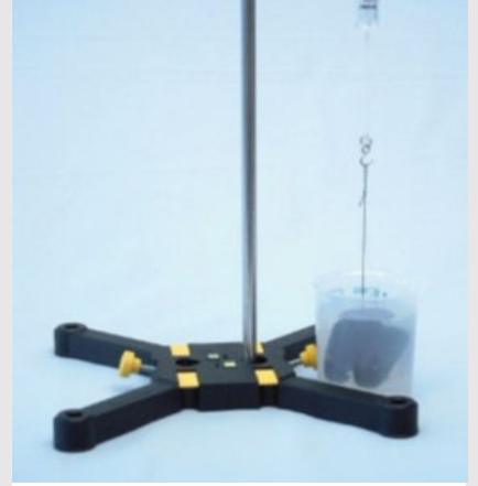
Determination of the weight forces in water F_{W,Water}
