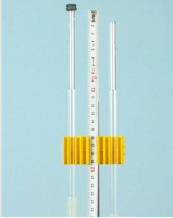
Place the rubber cap on the U-tube
