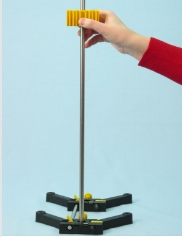
Attach the glass tube holder to the support rod
