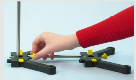
Fastening with the aid of the screw plug
