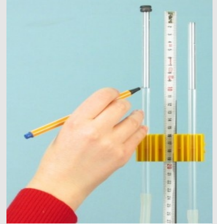
Marking the water level
