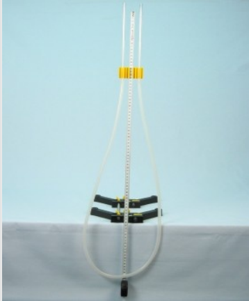
Experimental setup for the investigation of Boyle-Marriott's law
