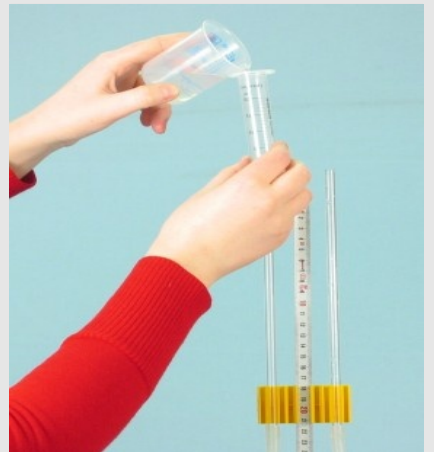
Fill U-pipe with water
