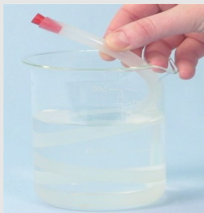
Press the rubber plug into the hose
