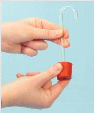
Put the glass tube into the stopper
