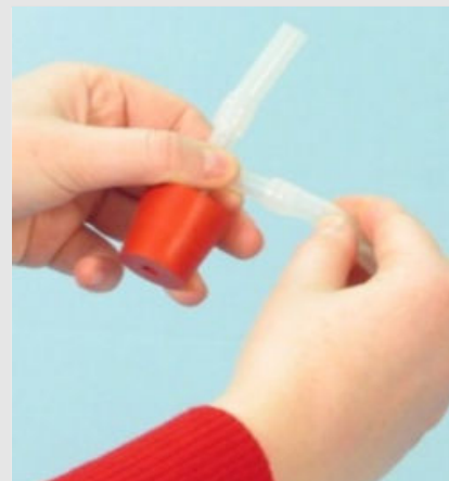
Connect the silicone hose to the ends of the T-piece.
