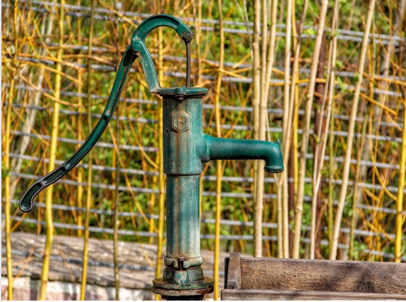
Garden pump for pumping water from a well
