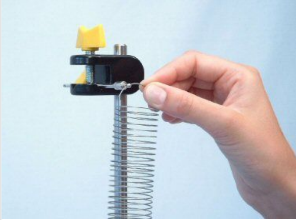
Hook the coil spring into the retaining bolt
