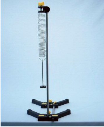
Test setup of the coil spring pendulum
