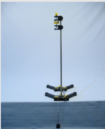
Experimental setup for the investigation of a mathematical pendulum
