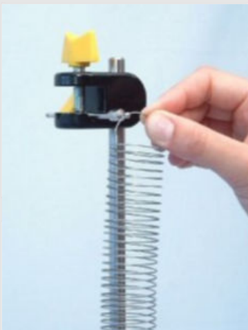
Holding pin with spring in the boss head
