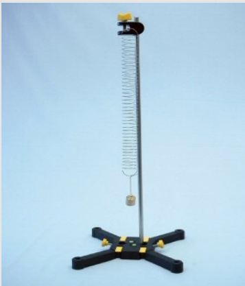
Experimental setup for determining the natural frequency of the spring pendulum
