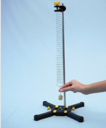
Deflection of the spring pendulum
