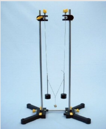
Experimental setup for the investigation of coupled pendulums
