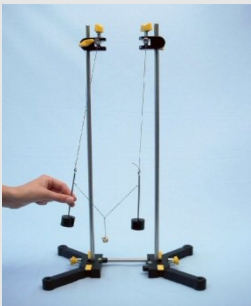
Deflection of the thread pendulum
