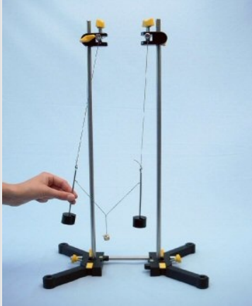
Deflection of the thread pendulum
