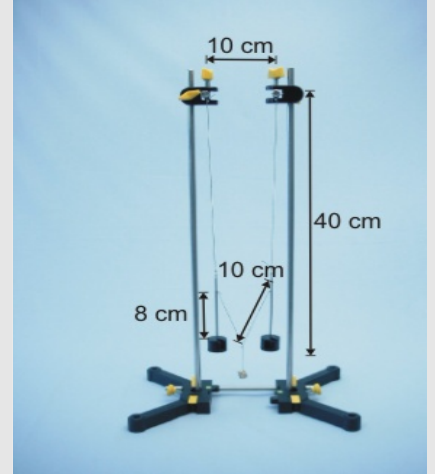
Build up of two equal thread pendulums
