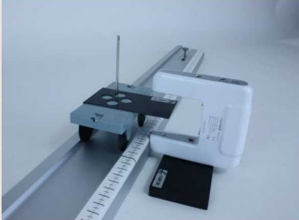
Connect adapter plate and light barrier
