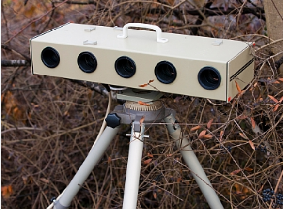
Measuring device for radar control
