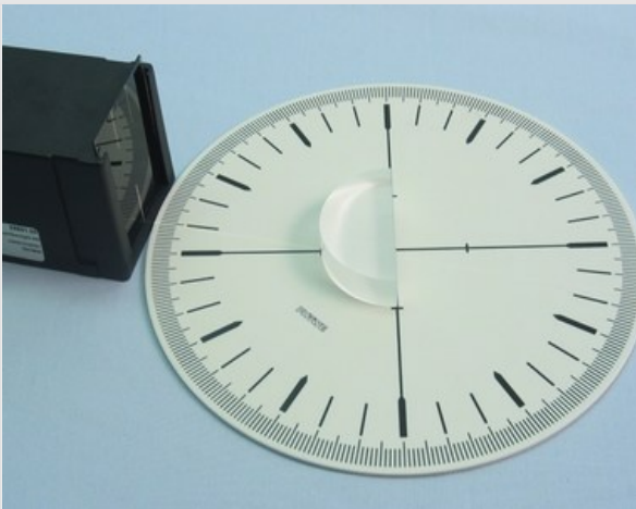
Refraction at the transition from glass to air
