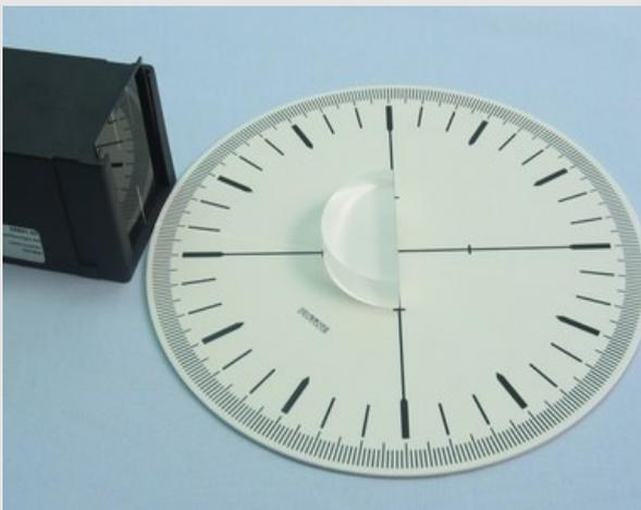
Refraction at the transition from glass to air
