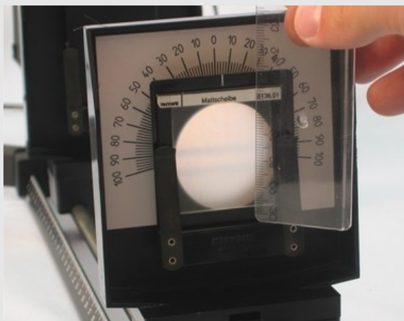
Measuring the size of the intermediate image on the ground glass screen
