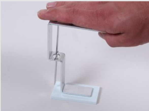
Touching the electroscope with the hand
