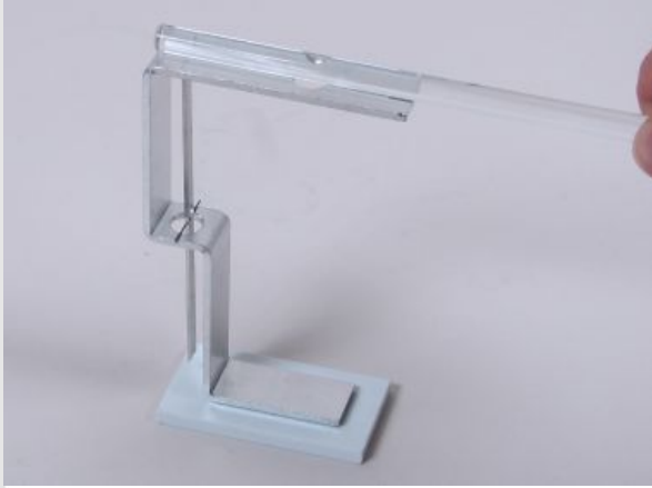
Passing the acrylic rod over the electroscope
