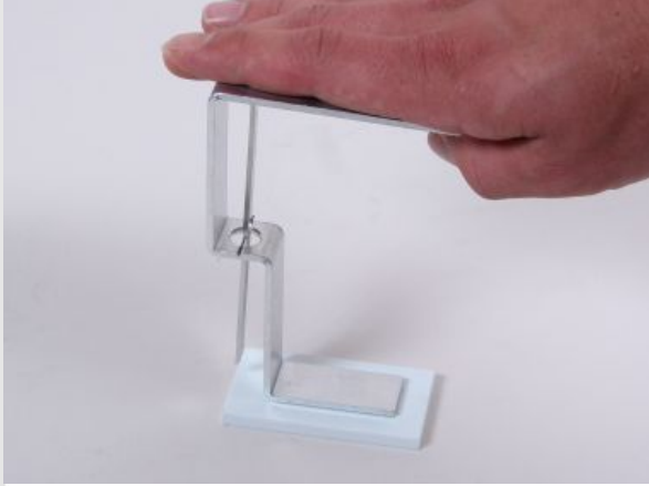
Touching the electroscope with the hand
