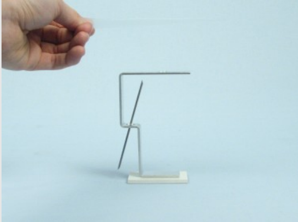
Approach charged transparent film to the electroscope
