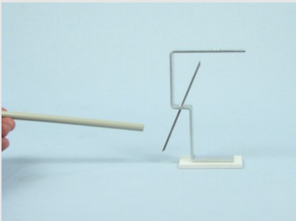
Bring the charged end of the rod close to the pointer
