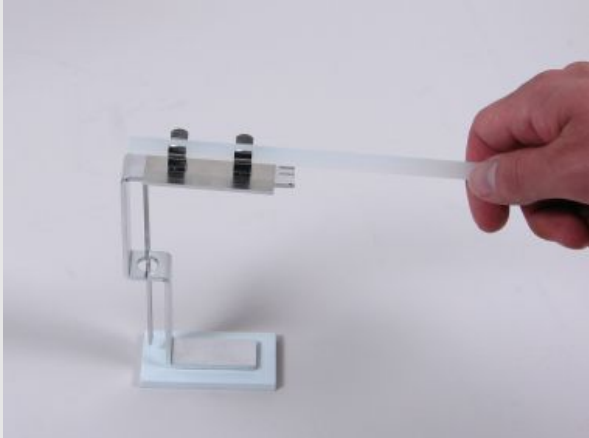
Connecting the electroscope and the influence plate
