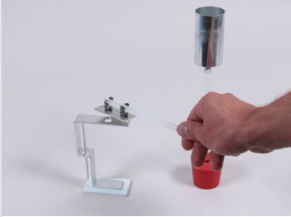
Alternately touching the Faraday cup and the electroscope
