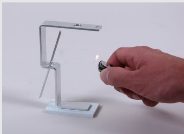
Heating the charged electroscope for ionisation
