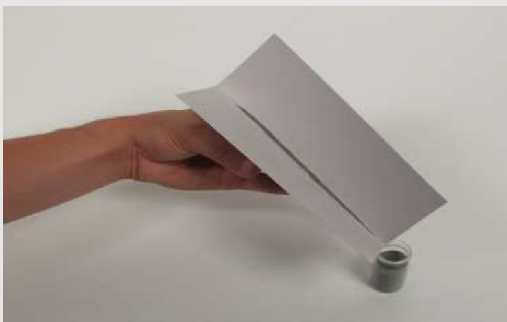
Procedure - Fill iron powder into powder dispenser
