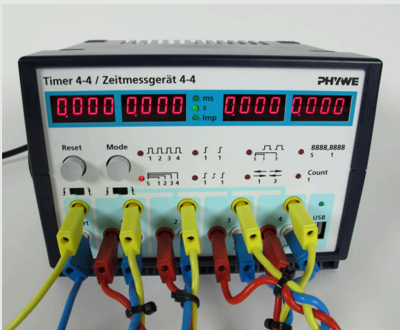
Connecting the light barriers
