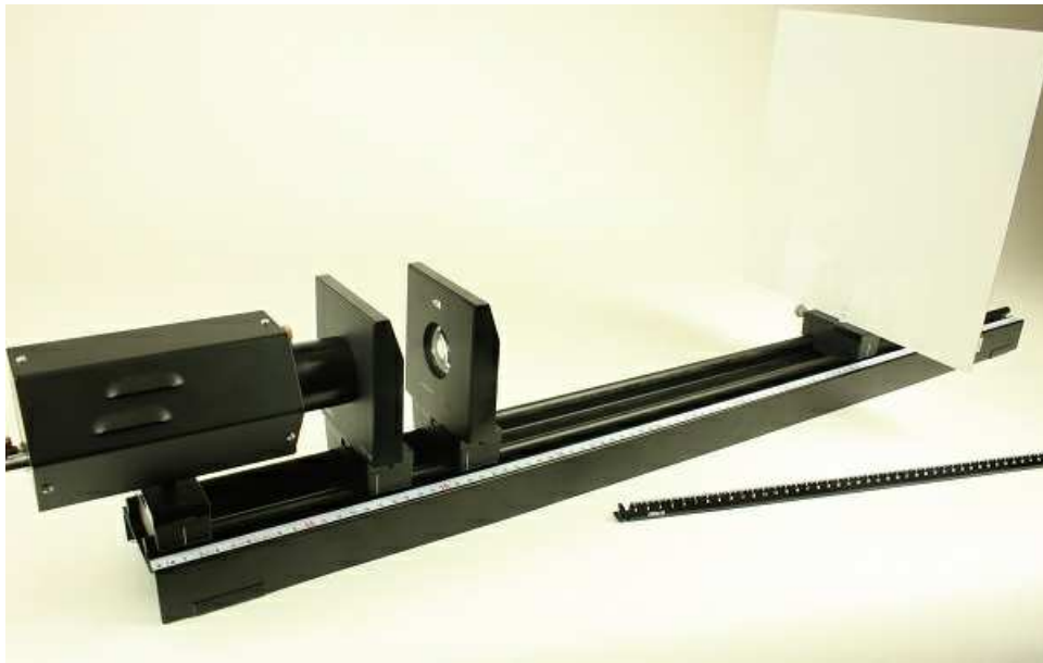
Fig. 2a: Setup for demonstration of the interim image
