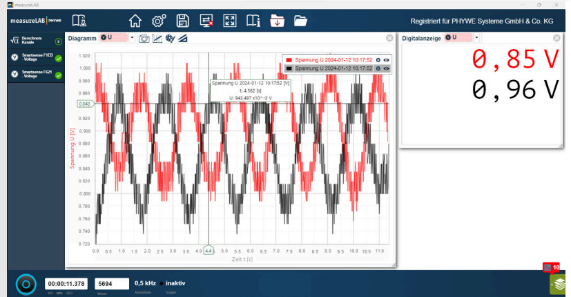
Figure 6: Representation of the deflection of both pendula for the “antiphase” oscillation as a function of time t.
