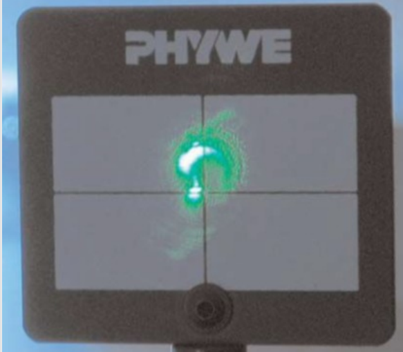
Bad laser tube alignment
