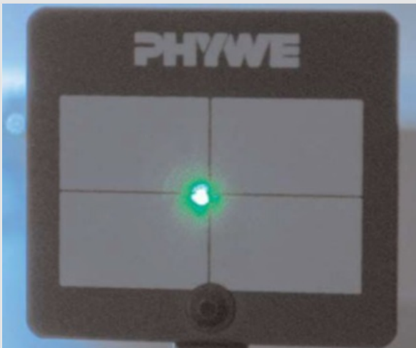
Good laser tube alignment
