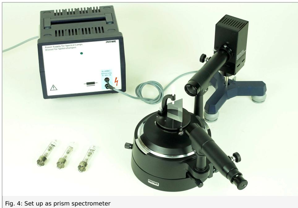
Fig. 4: Set up as prism spectrometer
