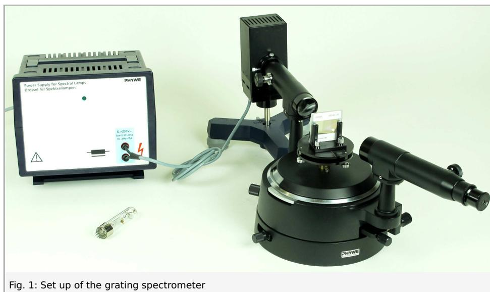
Fig. 1: Set up of the grating spectrometer
