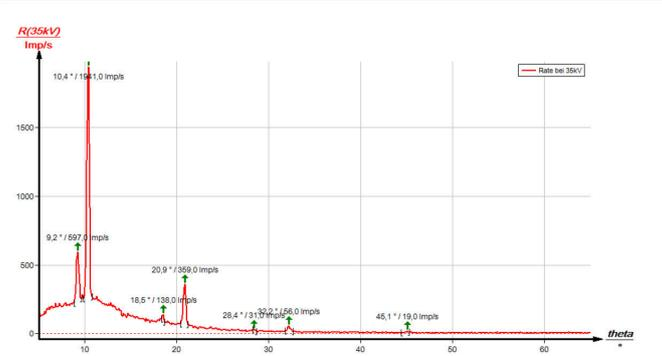
Fig. 9: X-ray spectrum of molybdenum; LiF monocrystal as the analyser
