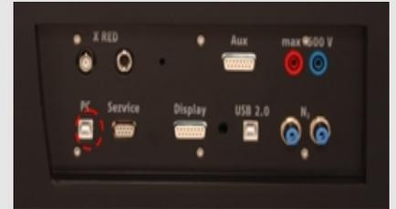
Fig. 5: Connection of the computer
