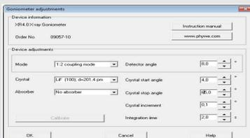
Fig 7: Settings of the goniometer (LiF crystal)
