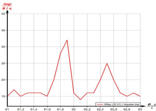
Fig. 11: Splitting of the  $K_{\alpha_1}$  and  $K_{\alpha_2}$  lines of molybdenum ( $n = 5$ )
