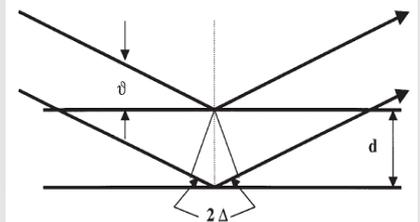
Fig. 2: Bragg scattering on a pair of lattice planes
