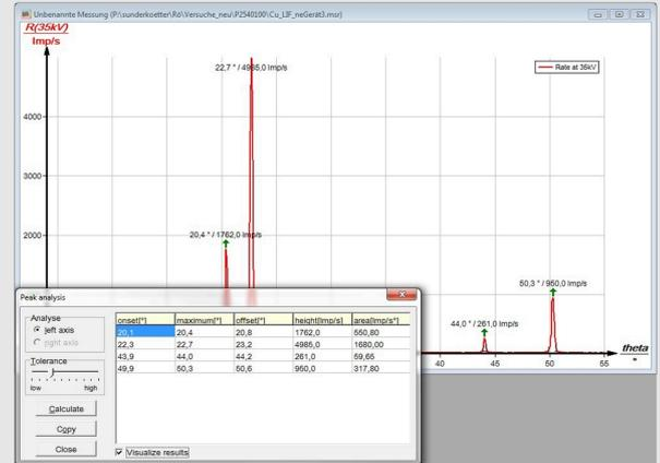
Fig. 12: Automatic peak analysis with "measure"
