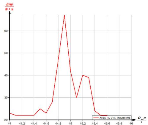
Fig. 10: Splitting of the  $K_{\alpha_1}$  and  $K_{\alpha_2}$  lines of molybdenum ( $n = 4$ )
