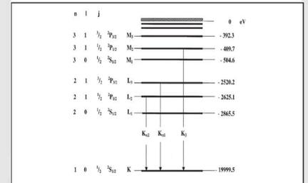
Fig. 1: Energy-level-diagram of molybdenum ( $Z = 42$ )
