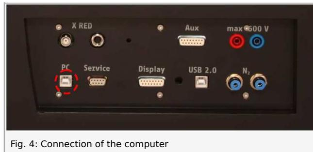
Fig. 4: Connection of the computer
