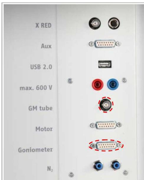
Fig. 2: Connectors in the experiment chamber
