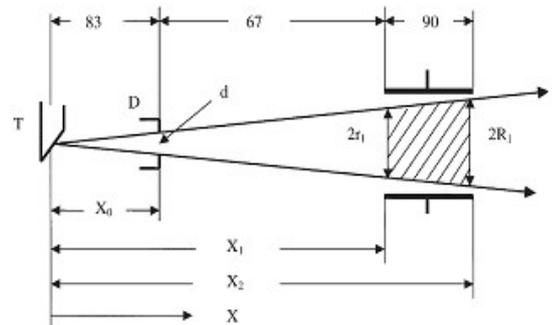
Fig. 6: Schematic representation of the beam geometry for the determination of the irradiated air volume (values in mm)
