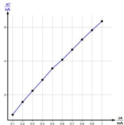
Fig. 8: Ionisation current  $I_C$  as a function of the anode current  $I_A$ ; Anode voltage  $U_A = 35 \text{ kV}$ ; Capacitor voltage  $U_C = 500 \text{ V}$ ; Diaphragm tube  $d = 5 \text{ mm}$
