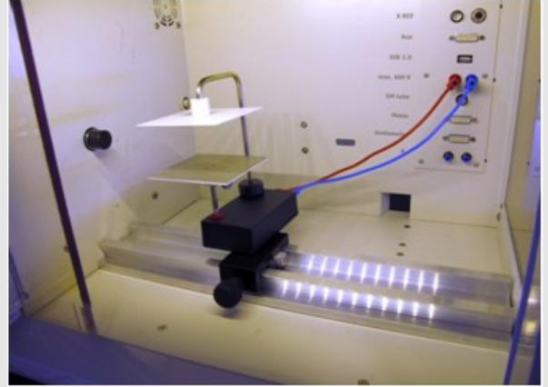
Fig. 5: Set-up and wiring of the capacitor plates inside the experiment chamber
