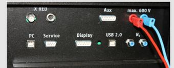
Fig. 2: Connection of the X-ray unit
