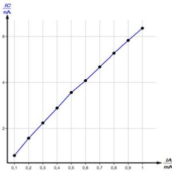
Fig. 8: Ionisation current  $I_C$  as a function of the anode current  $I_A$ ; Anode voltage  $U_A = 35$  kV; Capacitor voltage  $U_C = 500$  V; Diaphragm tube  $d = 5$  mm
