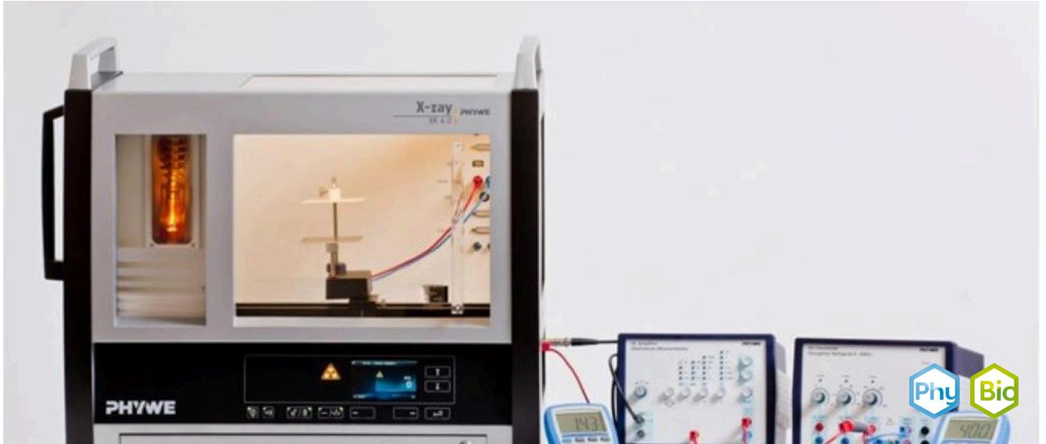
The goal of this experiment is to investigate the principle behind radiative dosimetry.
