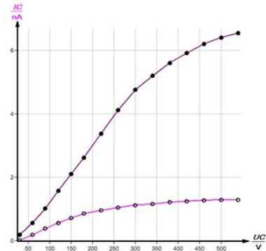
Fig. 7: Ionisation current  $I_C$  as a function of the capacitor voltage  $U_C$  X-ray tube:  $U_A = 35$  kV;  $I_A = 1$  mA, Curve A: diaphragm tube  $d = 5$  mm, Curve B: diaphragm tube  $d = 2$  mm
