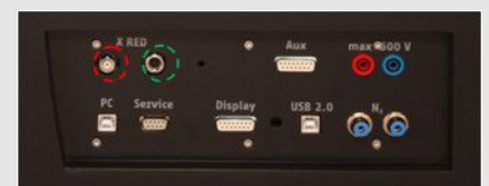
Fig. 2: Connection of the multi-channel analyser
