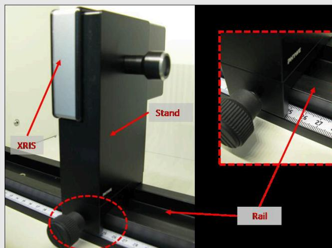
Fig. 1: Set-up of the XRIS
