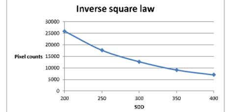
Fig. 10: Pixels counts in function of the SDD for same power and kV settings.
