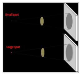
The relation between the detector pixels size (d), the focal spot size (s) and the system resolution (R) can be simplified with this formula:
