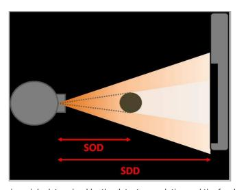
The resolution of an X-ray system is mainly determined by the detector resolution and the focal spot size resolution.
