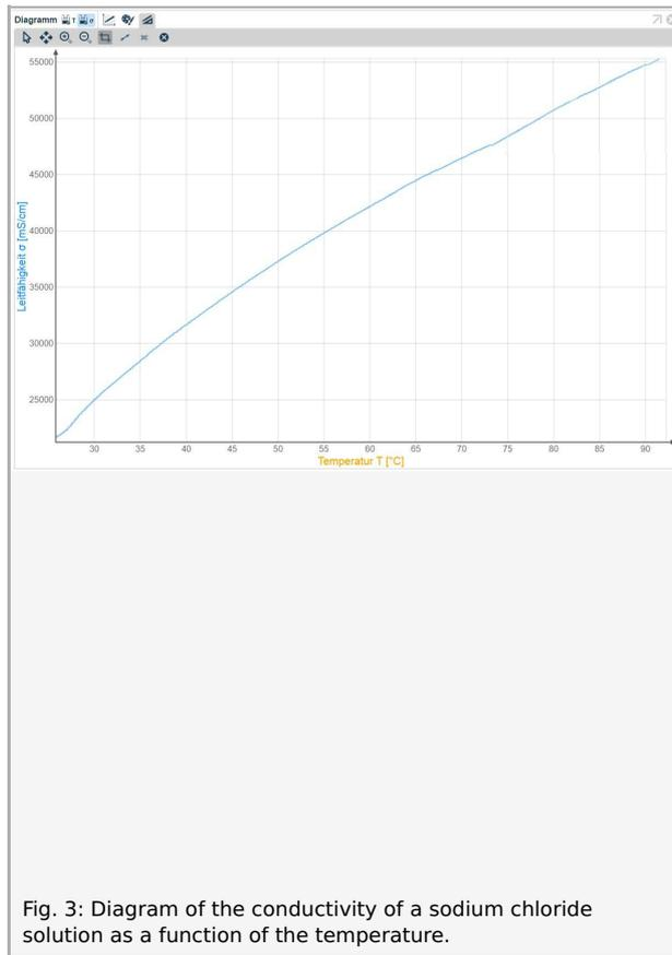
Fig. 3: Diagram of the conductivity of a sodium chloride solution as a function of the temperature.
