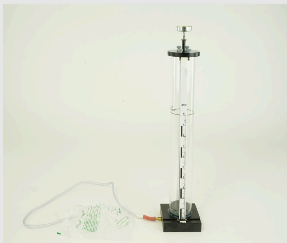
Setup of the gasometer
