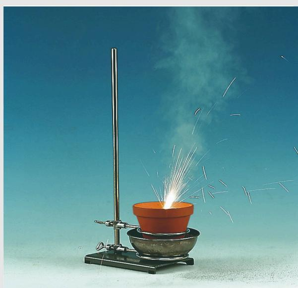
Thermite reactions have many uses. Thermite is not an explosive. It operates by exposing a very small area to extremely high temperatures. This can be useful to cut through metal or weld metal.
