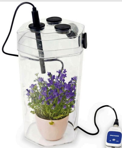
Experimental setup with reaction chamber, plant and sensor
