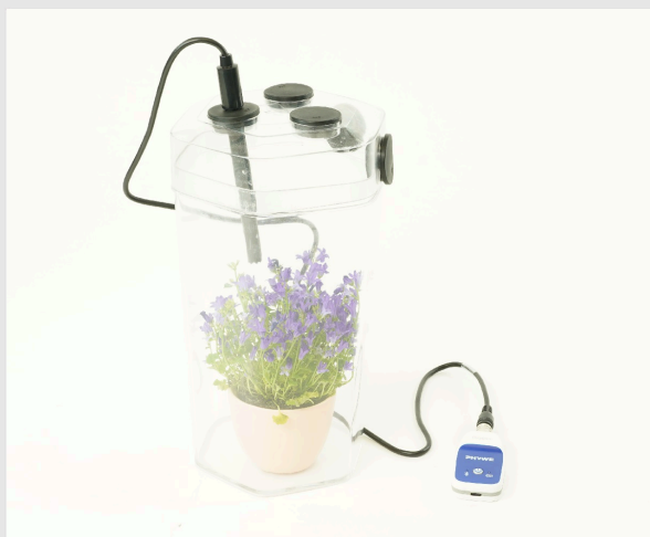
Experimental setup with reaction chamber, plant and sensor
