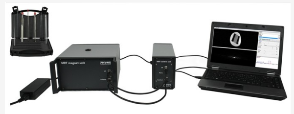
Fig. 11: Set-up of the MRT training unit
