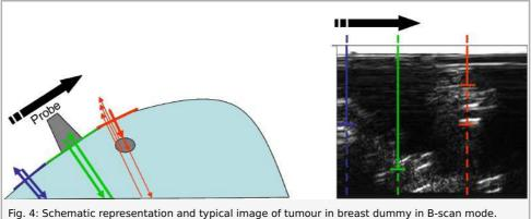
Without a scanner, only dept measurements give significant results. For lateral information the beam must be mechanically or electronically scanned over the area of interest. The most clinical ultrasound equipment use phase array electronic scanning method. The probe is fixed and the ultrasound beam scans the object by varying the incident angle.
