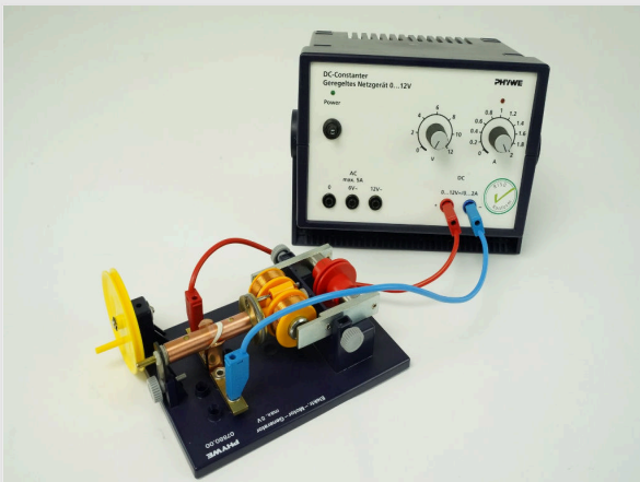
Electric motor connected to voltage source
