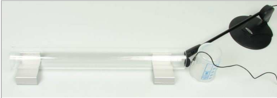
Fig. 4: The earphone and microphone in front of the open glass tube
