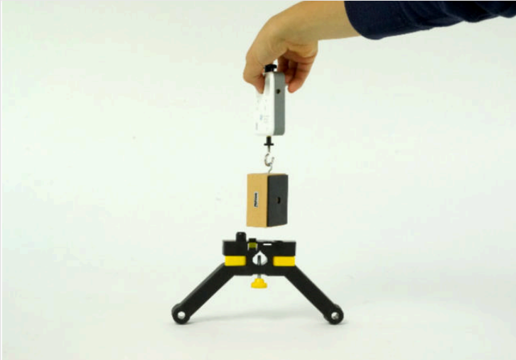
Measurement of the weight force of the friction block
