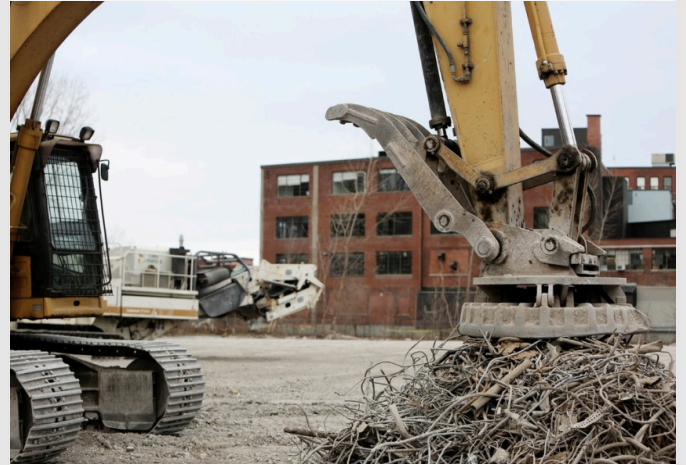
Electromagnet on an excavator
