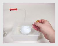
Carefully ignite the petrol in the evaporating dish and open the tap of the dropping funnel.
