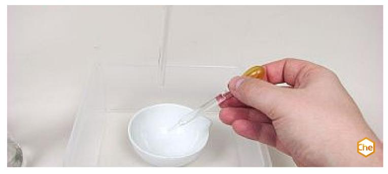
In this student experiment, the model of a fire extinguisher is reproduced. Here, the carbon dioxide (represented by sodium carbonate and hydrochloric acid) forms a foam with washing-up liquid, which is sprayed onto burning petrol and the flame goes out (by displacing the oxygen).
